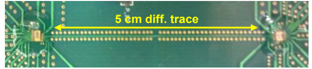
Fig. 8. Top view of the test board with separate TX/RX connected with a 5-cm FR-4 differential trace.
