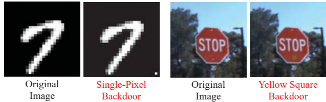
Figure 5: Original images of MNIST digit "7" and US "stop sign", and their respective backdoored images.
