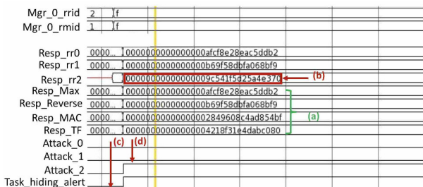
Fig. 5: Simulation snapshot of the FPGA-based reconfigurable system state when task hiding attack is launched in rr2 . (a) expected responses of registered users for a given challenge sent by SAM; (b) response of the hardware task configured in rr2 does not match the response of any registered user; (c) task hiding alert is asserted; (d) SAM determines that the attack occurs in rr2 .
