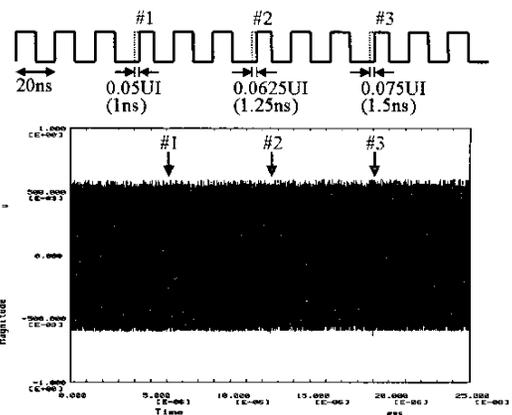
Figure 20 Digitized Waveform of Edge Shifted Clock
