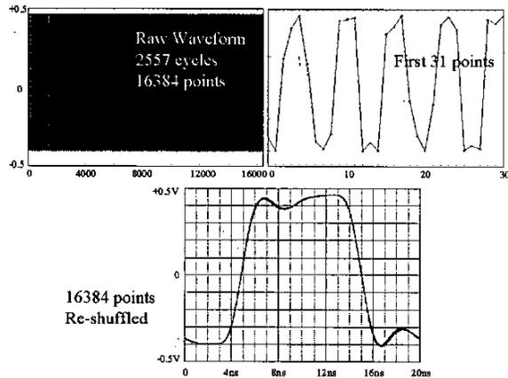
Figure 22 Digitized Waveform of 50MHz Clock
