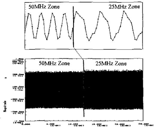
Figure 13 Digitized Waveform of On-the-fly Clock Change
