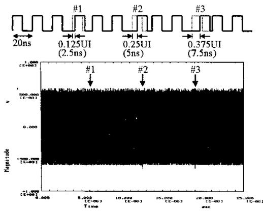
Figure 18 Digitized Waveform of Pulse Shifted Clock
