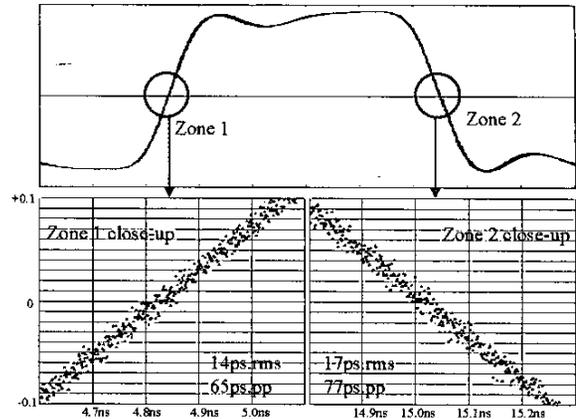
Figure 24 Rising Edge/Falling Edge Fluctuation
