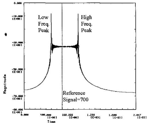
Figure 6 Spectrum of the Changing Frequency Signal
