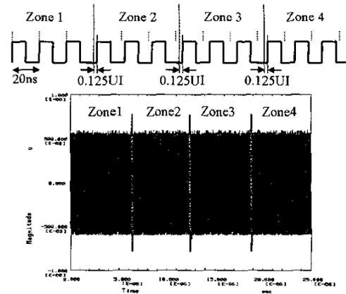
**Figure 16** Digitized Waveform of Phase Shifting Clock
