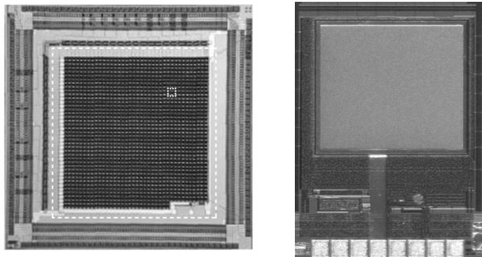
**Figure 7.4.7:** Micrograph of the retina implant chip (left) with indication of the sawing area with the test circuitry outside (dashed line) and a pixel cell (dotted line), as well as the TFC miniature imager chip (right).
