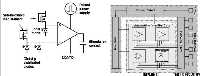
Figure 7.4.3: Circuit schematic of the pixel cell of the sub-retinal implant (left) and layout schematic (right) of the chip, indicating the chip section to be implanted (light grey) and the test circuit periphery to be removed after on-chip testing (dark grey).
