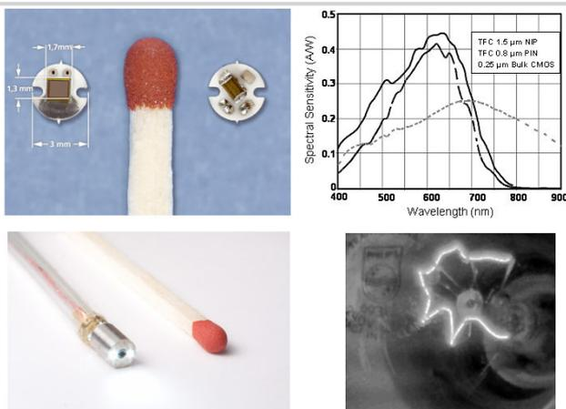
Figure 7.4.5: Photographs of the miniature imager chip mounted onto a special ceramic carrier (top; left) and of the fully assembled miniature endoscope (bottom; left); spectral sensitivities of the NIP and PIN  $\alpha$ -Si photodiodes in comparison to bulk silicon diodes (top; right); image of a 100W light bulb taken with the miniature endoscope indicating the high dynamic range (bottom; right).
