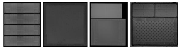
Fig 3 Both homogeneous and heterogeneous integration are demonstrated; from left to right, homogeneous 1x4, homogeneous 1x1, heterogeneous 1+1, heterogeneous 1+2. [8]
