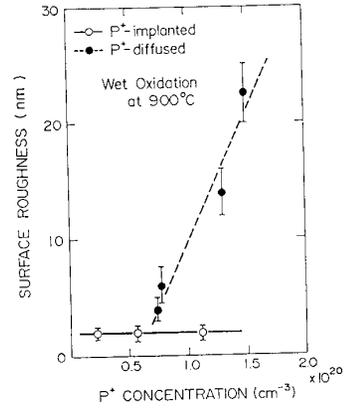
Fig.4 Surface roughness of gate oxide as a function of P<sup>+</sup> concentration.
