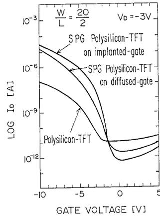
Fig.6 Subthreshold characteristics of fabricated p-ch TFTs.
