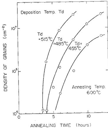
Fig.2 Density of grains as a function of annealing time.
