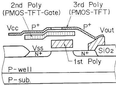
Fig.1 Cross-sectional view of inverter in stacked-CMOS SRAM cell.
