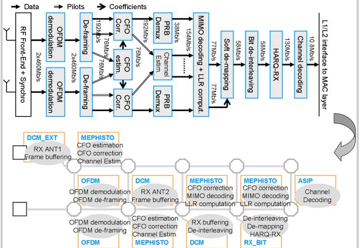
Figure 15.3.4: 3GPP-LTE 4x2 MIMO scheme on the receiver side.
