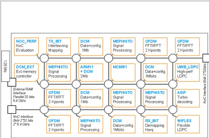
Figure 15.3.1: Structure and processing cores.
