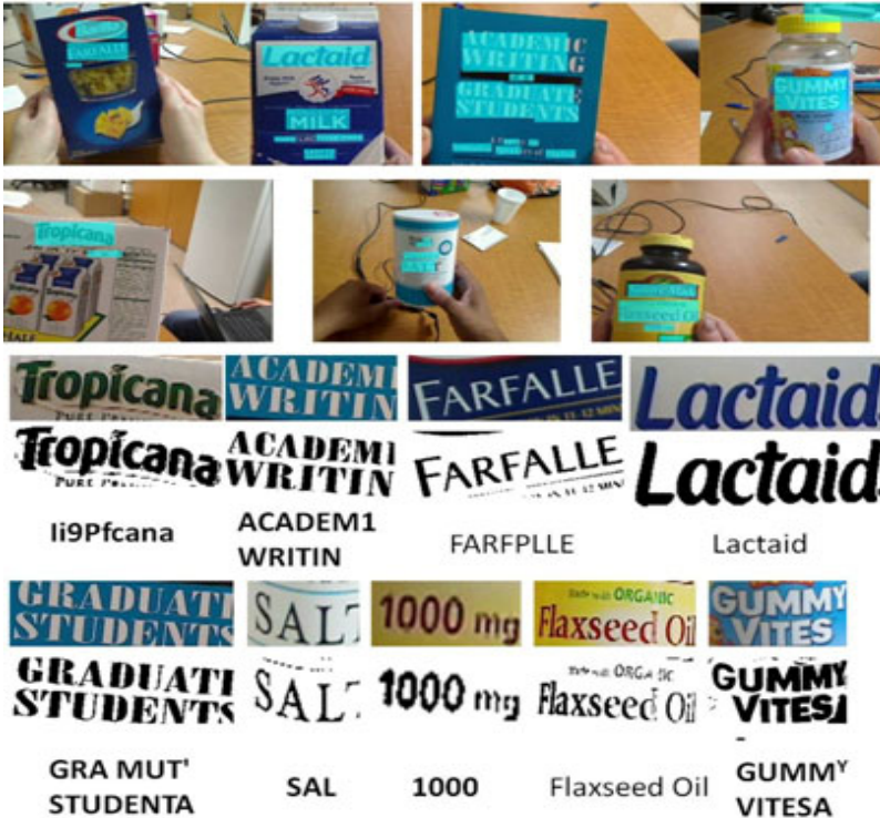
Fig. 10. The top two rows present some results of text localization on the blind-captured dataset, where localized text regions are marked in cyan. The bottom rows show two groups of enlarged text regions, binarized text regions and word recognition results from top to down.
