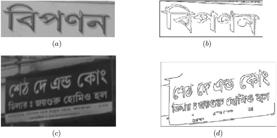
Fig. 1. (a) and (c) two original (gray level) images (or its part) from our database of natural scenes; (b) and (d) Canny edges of the images in (a) and (c)
