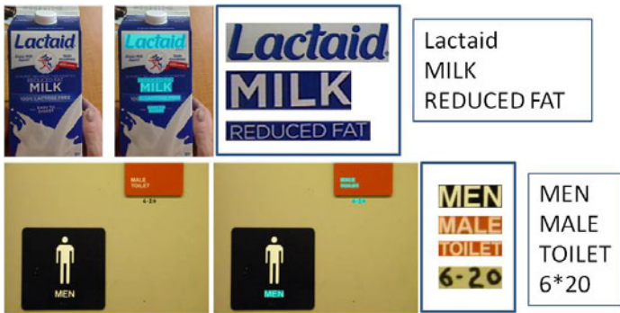
Fig. 1. Two examples of text localization and recognition from camera captured images. Top: a milk box; Bottom: a male bathroom. From left to right: camera-captured images, localized text regions (marked in cyan), text regions, and text codes recognized by OCR.
