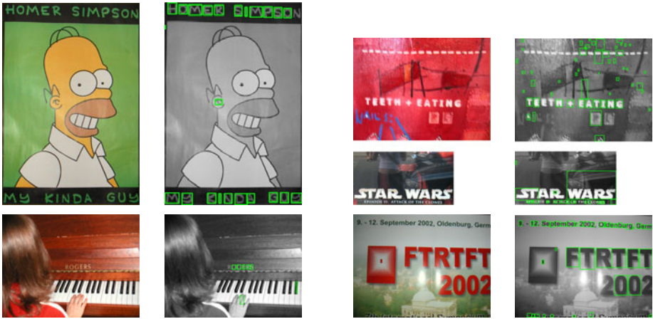
Fig. 18. A few samples from ICDAR 2003 image database of natural scenes on each of which performance of the proposed algorithm is poor. Portions identified as texts are marked by green colored rectangular boundaries.
