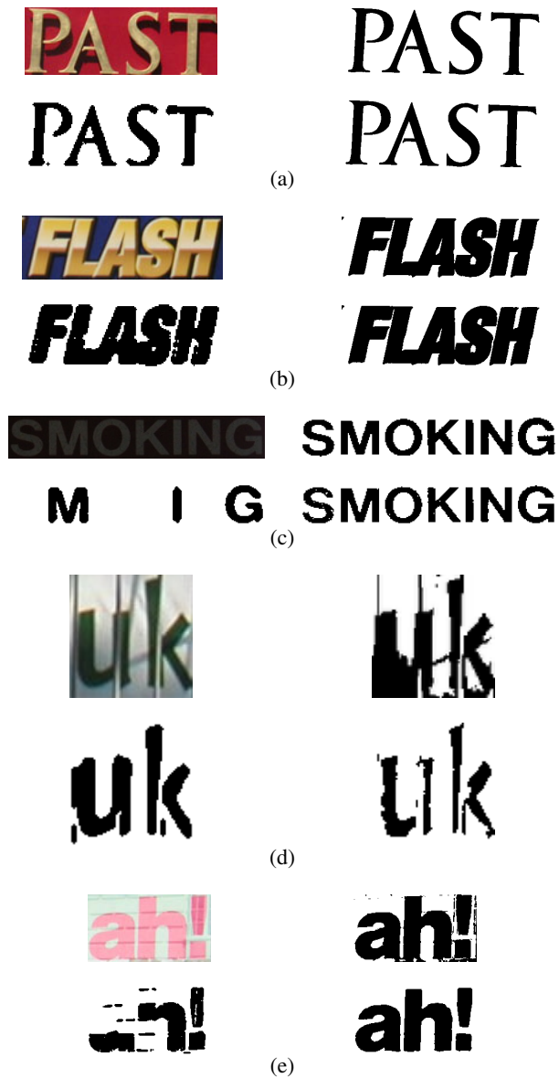
Fig. 6. Comparison of segmentation results in other cases. Top left: original image; top right: Otsu's method; bottom left: the method in [7]; bottom right: the proposed method.
