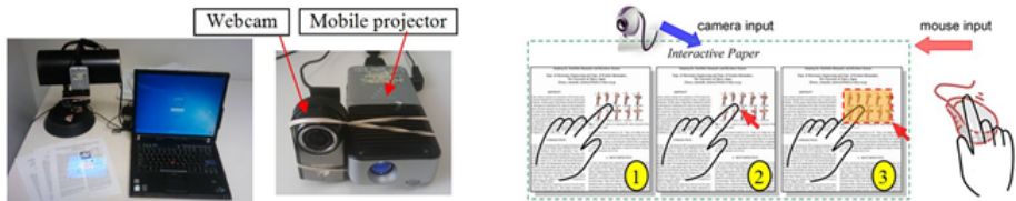
Fig. 7. (left) MixPad interface prototype, (middle) Close-up of the camera-projector unit, and (right) steps to select a picture portion: (1) roughly pointing a finger to a region, (2) mouse cursor being projected to where the fingertip is, and (3) Drawing a mouse marquee gesture to select a region at fine granularity. Excerpt from Liao et al.[37].
