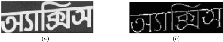
Fig. 8. (a) A sub-image of the image shown in Fig. 5(a); (b) skeleton-like representation of the object in (a) formed by the pixels in its \langle T \rangle
