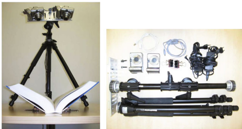
Fig. 1. A prototype scanning rig, consisting of standard tripod hardware and consumer digital cameras. The rig is portable and can be operated anywhere using a laptop computer.
