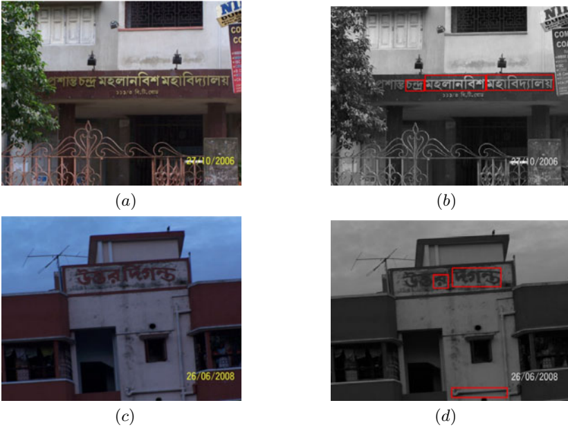
Fig. 16. (a) and (c): Two samples from our image database. In (b) a few words of (a) remain undetected since these have got connected in the Canny edgemap with adjacent non-text components; in (c) the text portion is dirty due to fungus. The false detection in (d) is due to the presence of a strong linear component.
