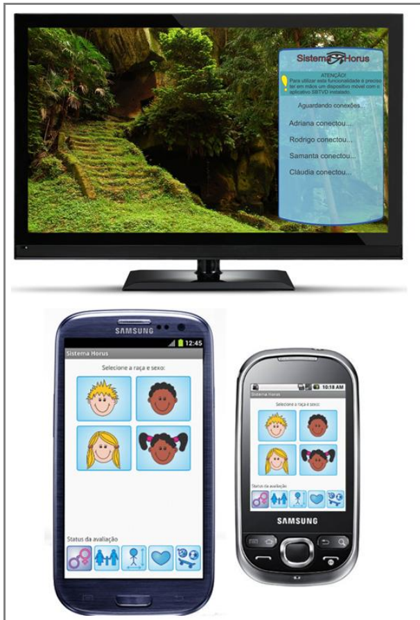
Figure 7: Primary screen (top) showing instructions and who's connected and second screen application (bottom) in many devices
