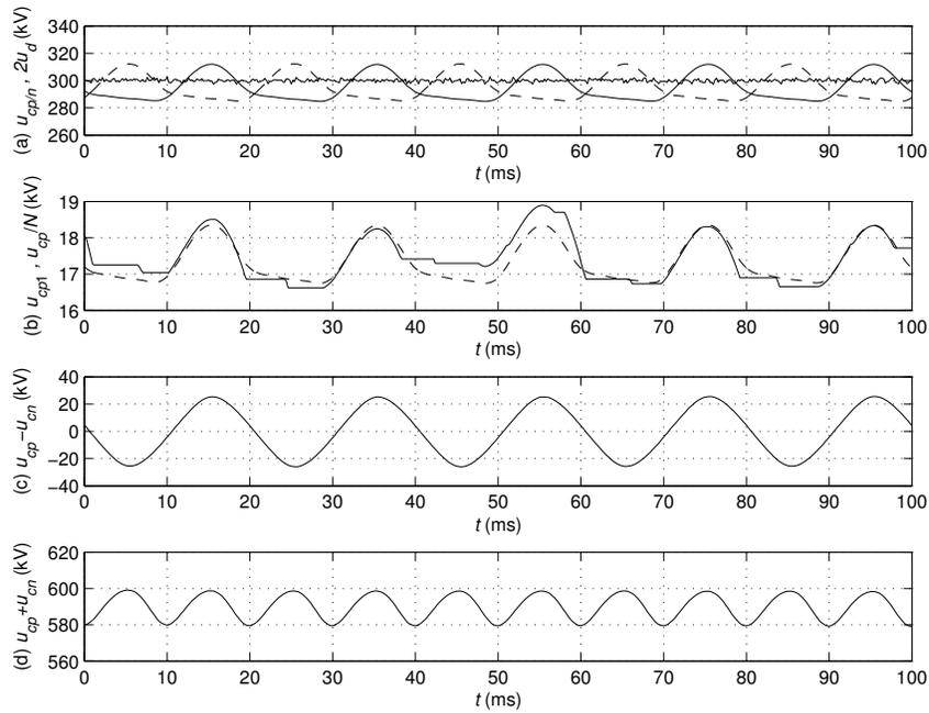
**Figure 3:** (a) Sum cell voltages for positive (solid) and negative (dashed) arms as well as two times the mean direct voltage (noisy due to switching harmonics). (b) Voltage of cell 1 in the positive arm with the mean cell voltage overlaid (dashed). (c) Differential-mode sum cell voltage. (d) Common-mode sum cell voltage.
