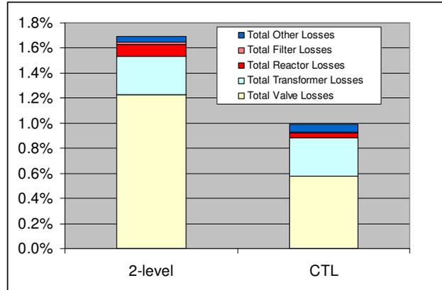
Figure 5: Typical converter losses.
