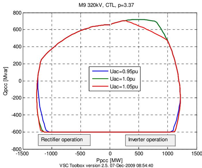
Figure 4: Example of active- and reactive-power capability.
