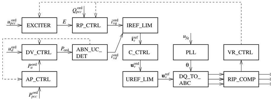
**Figure 7: Block diagram of the upper-level control.**
