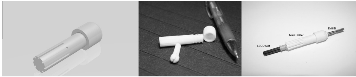
Fig. 2. The 3D design of the chuck (left) and the 3D printed one (right).
