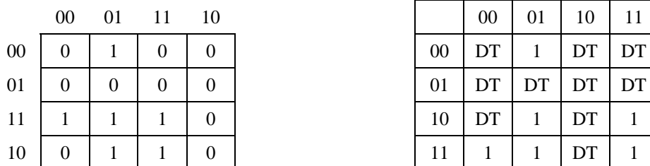
Figure 2. Example of the transformation of 2-level logic minimization into the simplified configuration compression problem. The Karnaugh Map (left) of the circuit is transformed into the configuration to be compressed (right). “DT” indicates don’t touches in the configuration.
