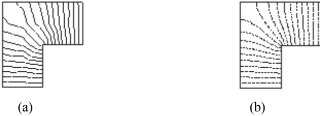
Figure 12.14 (a) Equipotential ( \Omega ) lines for the coarse mesh of Figure 12.11. (b) Equipotential ( \Omega ) lines for a dense mesh.
