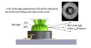
Figure 5: Optical Ray trace with diverter
