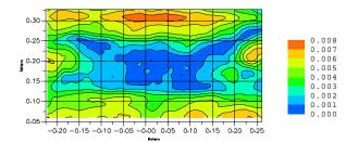
Figure 8: Measured Color uniformity Δu'v'
