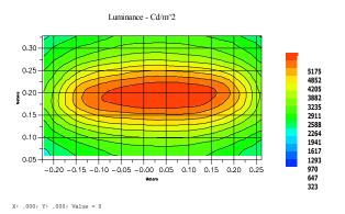
Figure 7: Measured Brightness uniformity
