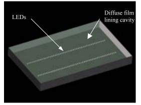
Figure 1: Typical RGB Layout within reflective cavity
