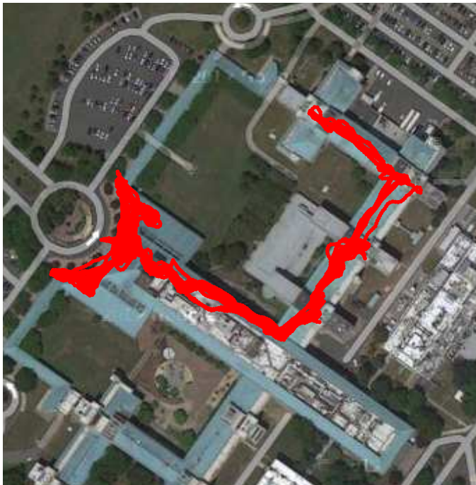
Fig. 6. Jointly reconstructed trajectories of three different phones (from Figs. 3, 4 and 5). Joint SignalSLAM was run with a WiFi- and Bluetooth-based kernel computed using measurements from all the phones at once.
