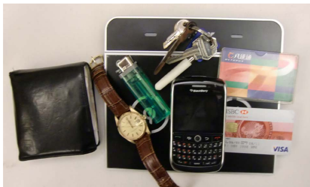
Fig. 5. A photograph of a wireless charging pad with a variety of compatible and noncompatible items.
