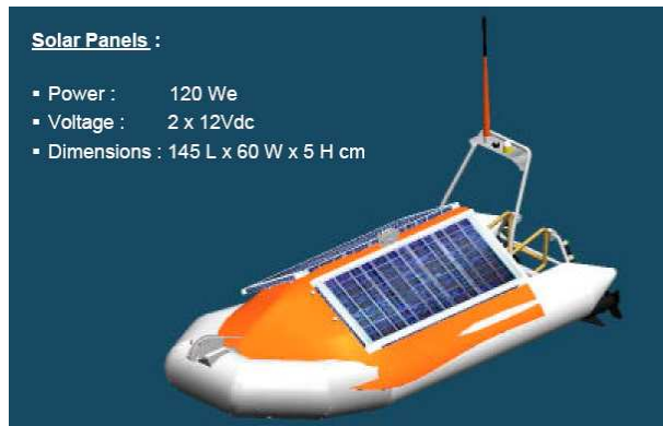
Basil-II with solar panels
