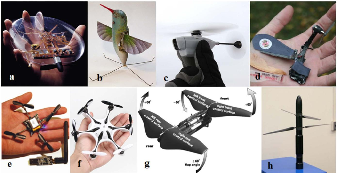
**Fig. 8.** Different types of NAVs, (a) fixed wing [133], (b) flapping wing [134], (c) helicopter [135], (d) monocopter [136], (e) quadrotor [137], (f) hexacopter [138], and (g and h) unconventional [139,140].
