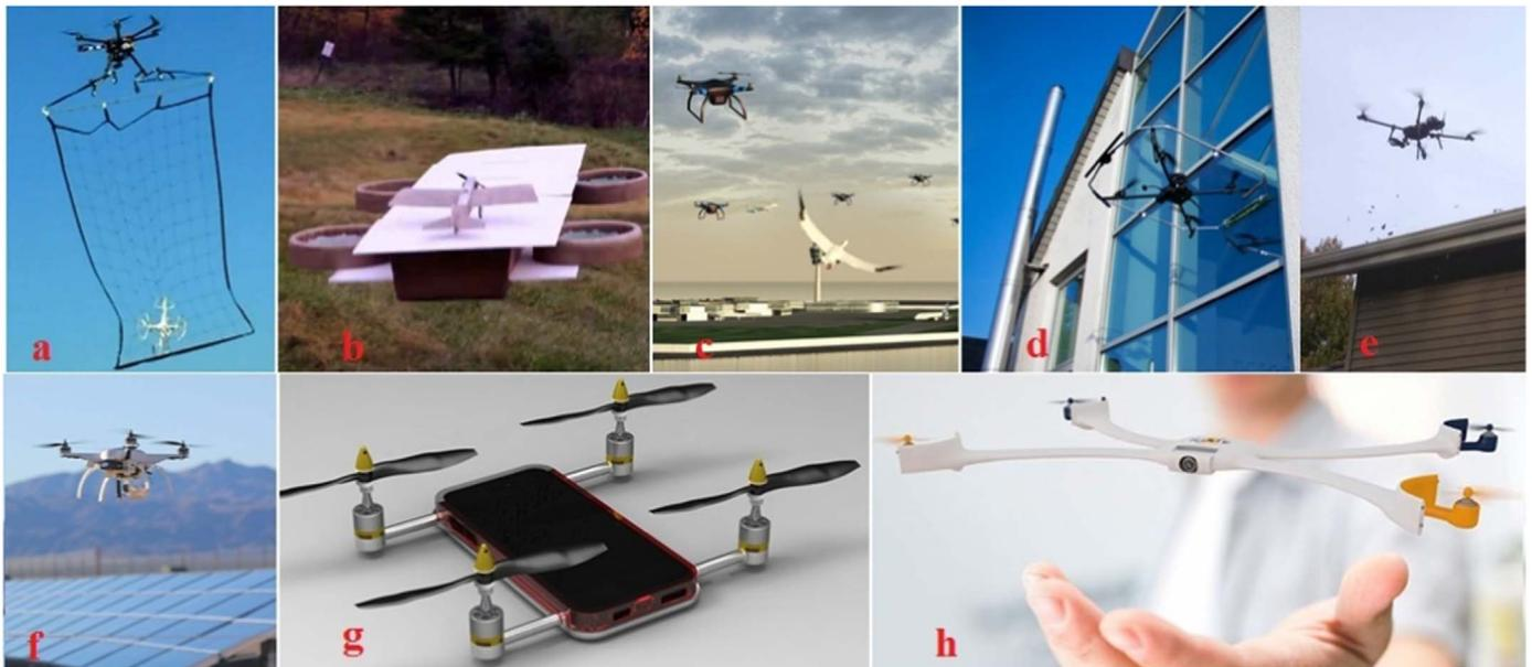
**Fig. 21.** Drones' miscellaneous applications, (a) anti-drones [216], (b) runway drone [217], (c) drones which scare birds away from airport runways [218], (d) windows cleaning drones [219], (e) gutters cleaning drones [221], (f) solar panels cleaning drones [222], and (g and h) hobby drones [220,223].
