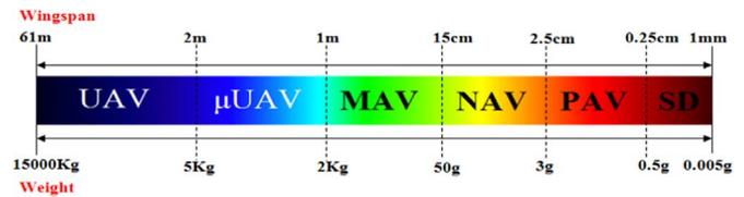
Fig. 1. Spectrum of drones from UAV to SD.
